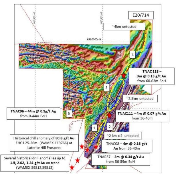
**Fig.10**: Summary of Target Trends prioritised from air magnetics interp. and drill data: Red stars within E20/714 are results from historical RAB or Air Core drilling which support recent drill testing. Red stars immediately to the south west of E20/714 reporting one metre intervals in historical regolith drilling.
